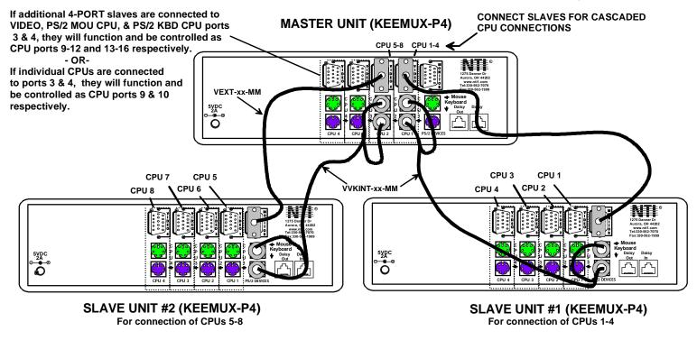
Figure 6- Cable connections for cascading
